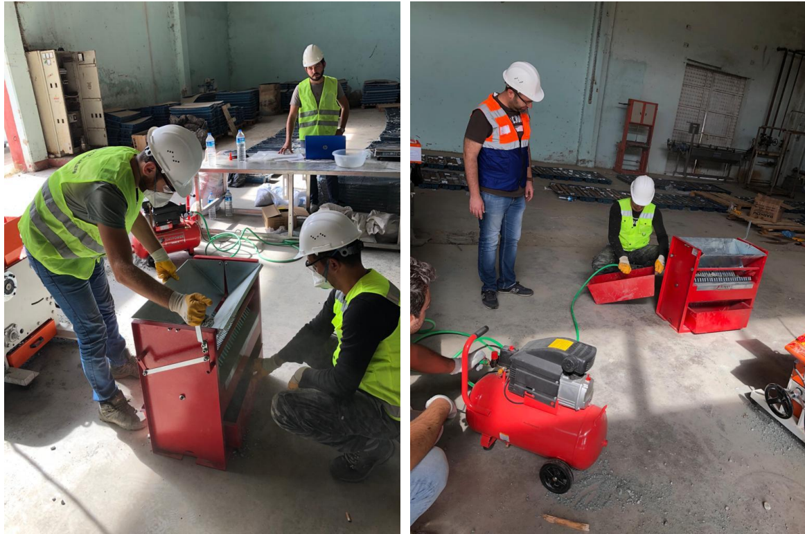
Figure 27. Steps of sample preparation: Equipment in core shed (Top Left), Crushing (Top Right), Splitting (Bottom Left), Cleaning (Bottom Right).
